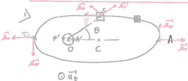
$$\vec{L}_O = m \vec{r} \wedge \vec{v} = m r^2 \vec{u}_r \wedge (-v_s \cos \theta \vec{u}_r + v_s \sin \theta \vec{u}_\theta)$$
